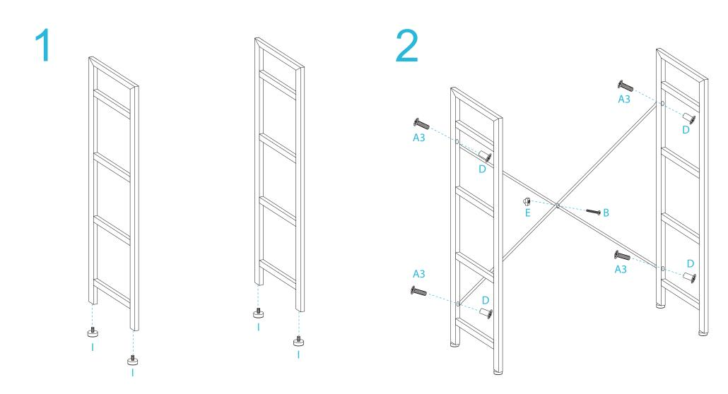
Attach 4x feet (I) to the bottoms of the side panels.
